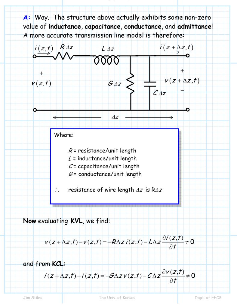
Dividing the first equation by  $\Delta z$ , and then taking the limit as  $\Delta z \rightarrow 0$ :
