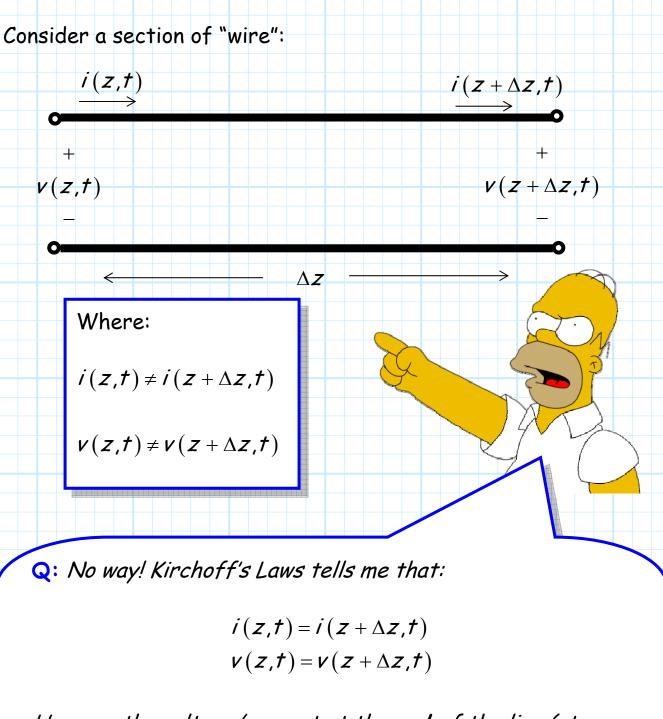
How can the voltage/current at the **end** of the line (at  $z + \Delta z$ ) be **different** than the voltage/current at the **beginning** of the line (at z)??
